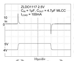
Transient Line Regulation with 4.7µF MLCC Capacitor
