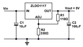
Figure 1 Basic Adjustable Regulator with 5V Output
