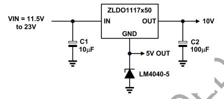
Figure 3 ZLDO1117 with Extended Output Voltage
